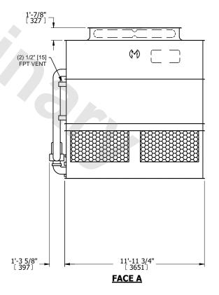
NO. OF SHIPPING SECTIONS **SHIPPING OPERATING** HEAVIEST SECTION 11520 lbs+ [5230] kg+ 13320 lbs+ [6045] kg+ 19880 lbs+ [9020] kg+ WEIGHT WEIGHT WEIGHT
