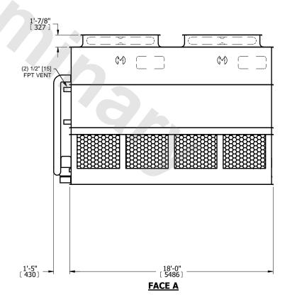
DRAWN BY: SLR NO. OF SHIPPING SECTIONS **SHIPPING** OPERATING HEAVIEST SECTION 19920 lbs+ [9040] kg+ 29780 lbs+ [13510] kg+ 17130 lbs+ [7775] kg+ WEIGHT WEIGHT WEIGHT
