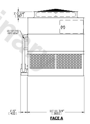
**SHIPPING OPERATING** HEAVIEST SECTION 12580 lbs+ [5710] kg+ 20090 lbs+ [9115] kg+ WEIGHT WEIGHT WEIGHT
