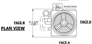
1'-1" [ 330 ] 1'-3/4" [ 324 ] 1'-10" [ 559 ] (2) 4" [100] BFW FLUID IN 5'-11 7/8" [ 1826 ] - (2) 4" [100] BFW FLUID OUT 9'-1 3/8" [ 2778 ] 1'-7 1/2" \* [ 495 ] - 1" [25] MPT MAKE-UP - 2" [50] FPT OVERFLOW
