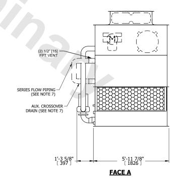
DRAWN BY: CAF NO. OF SHIPPING SECTIONS **SHIPPING** OPERATING HEAVIEST SECTION 2750 lbs+ [1250] kg+ 4270 lbs+ [1940] kg+ 2240 lbs+ [1020] kg+ WEIGHT WEIGHT WEIGHT
