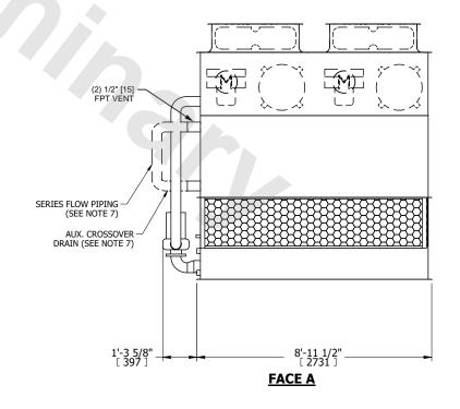
DRAWN BY: **SHIPPING OPERATING** HEAVIEST SECTION NO. OF SHIPPING SECTIONS 4600 lbs+ [2090] kg+ 6990 lbs+ [3175] kg+ 3930 lbs+ [1785] kg+ WEIGHT WEIGHT WEIGHT
