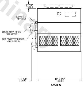
**SHIPPING** OPERATING HEAVIEST SECTION 9230 lbs+ [4190] kg+ 13910 lbs+ [6310] kg+ 7590 lbs+ [3445] kg+ WEIGHT WEIGHT WEIGHT
