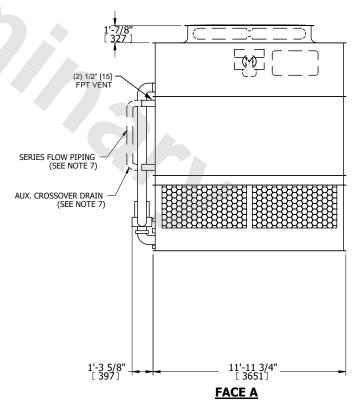
DRAWN BY: JLG NO. OF SHIPPING SECTIONS **SHIPPING** OPERATING HEAVIEST SECTION 16800 lbs+ [7625] kg+ 24480 lbs+ [11105] kg+ 15000 lbs+ [6805] kg+ WEIGHT WEIGHT WEIGHT
