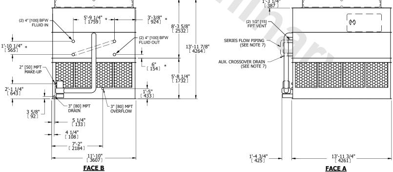
SHIPPING WEIGHT 16200 lbs+ [7350] kg+ OPERATING WEIGHT 26320 lbs+ [11940] kg+ HEAVIEST SECTION WEIGHT 13140 lbs+ [5965] kg+ NO. OF SHIPPING SECTIONS 2 DRAWN BY: JLG
