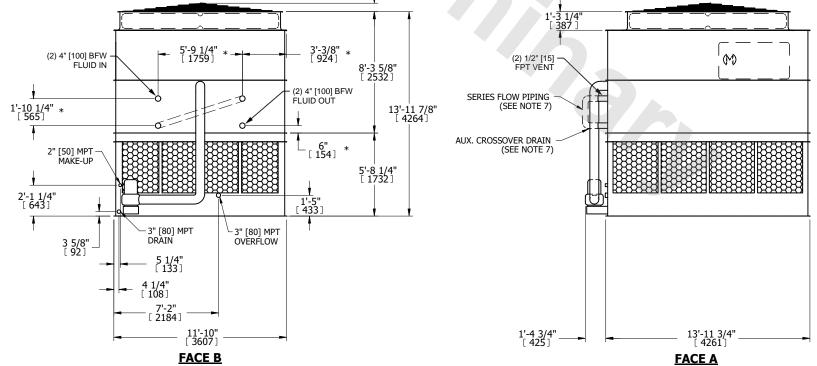
SHIPPING WEIGHT 16200 lbs+ [7350] kg+ OPERATING WEIGHT 26320 lbs+ [11940] kg+ HEAVIEST SECTION WEIGHT 13140 lbs+ [5965] kg+ NO. OF SHIPPING SECTIONS 2 DRAWN BY: JLG
