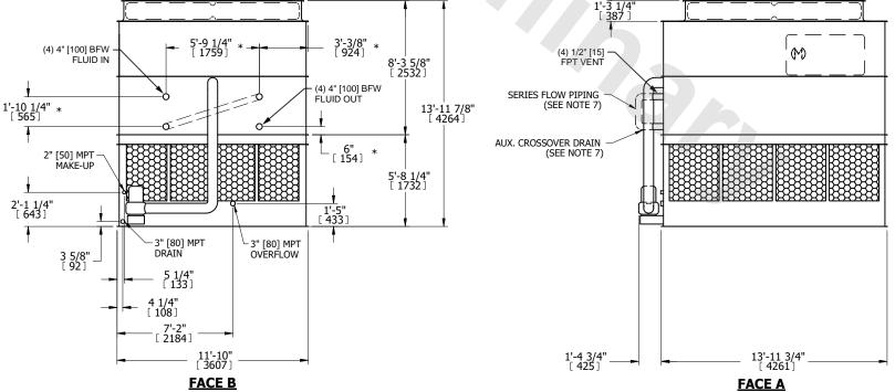
SHIPPING WEIGHT 16250 lbs+ [7375] kg+ OPERATING WEIGHT 26370 lbs+ [11965] kg+ HEAVIEST SECTION WEIGHT 13190 lbs+ [5985] kg+ NO. OF SHIPPING SECTIONS 2 DRAWN BY: JLG
