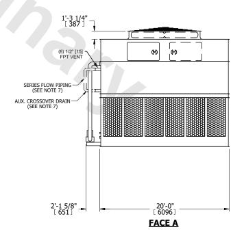
DRAWN BY: JLG **SHIPPING OPERATING** HEAVIEST SECTION NO. OF SHIPPING SECTIONS 59740 lbs+ [27100] kg+ 94160 lbs+ [42715] kg+ 25360 lbs+ [11505] kg+ WEIGHT WEIGHT WEIGHT
