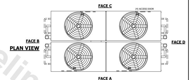
2'-6 3/8" \* [ 772] (16) 4" [100] BFW (16) 1/2" [15] M FLUID IN FPT VENT 10'-5 1/8' [ 3180 ] (16) 4" [100] BFW SERIES FLOW PIPING FLUID OUT 18'-7 3/8" 5674 (SEE NOTE 7) AUX. CROSSOVER DRAIN (SEE NOTE 7) 6" [ 154] 8'-2 1/4" [ 2494 ] 3'-10" [ 1168] (4) 2" [50] MPT -MAKE-UP 9'-4 1/2" [ 2858] (4) 3" [80] MPT 9'-5 1/2' [ 2883] 3 5/8' 1'-11 1/4" [ 591] 1'-11 1/4" 「591〕 5 1/8" [ 130] 9'-9 3/4' [ 2991] (4) 3" [80] MPT **FACE A FACE B**
