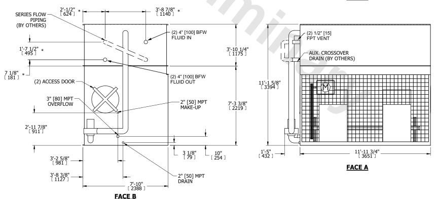
DRAWN BY: NO. OF SHIPPING SECTIONS **SHIPPING** OPERATING HEAVIEST SECTION 5870 lbs+ [2665] kg+ 9690 lbs+ [4400] kg+ 14730 lbs+ [6685] kg+ WEIGHT WEIGHT WEIGHT
