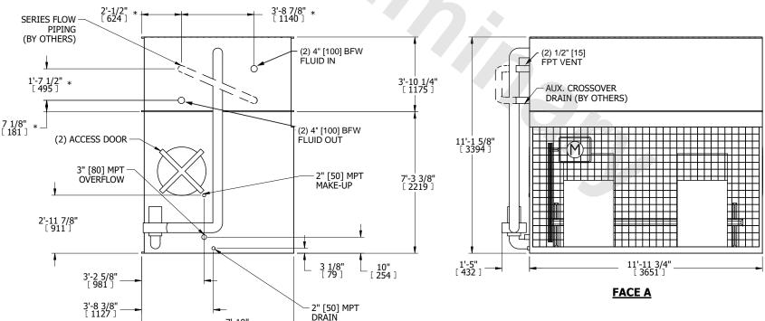
SHIPPING 9900 lbs+ [4495] kg+ OPERATING WEIGHT 14940 lbs+ [6780] kg+ HEAVIEST SECTION WEIGHT 5870 lbs+ [2665] kg+ NO. OF SHIPPING SECTIONS
