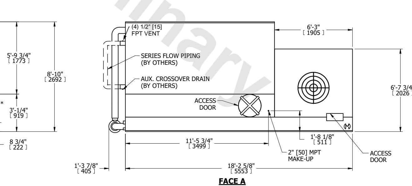
SHIPPING WEIGHT 16740 lbs+ [7595] kg+ OPERATING WEIGHT 24650 lbs+ [11185] kg+ HEAVIEST SECTION WEIGHT 16740 lbs+ [7595] kg+ NO. OF SHIPPING SECTIONS 1 DRAWN BY:
