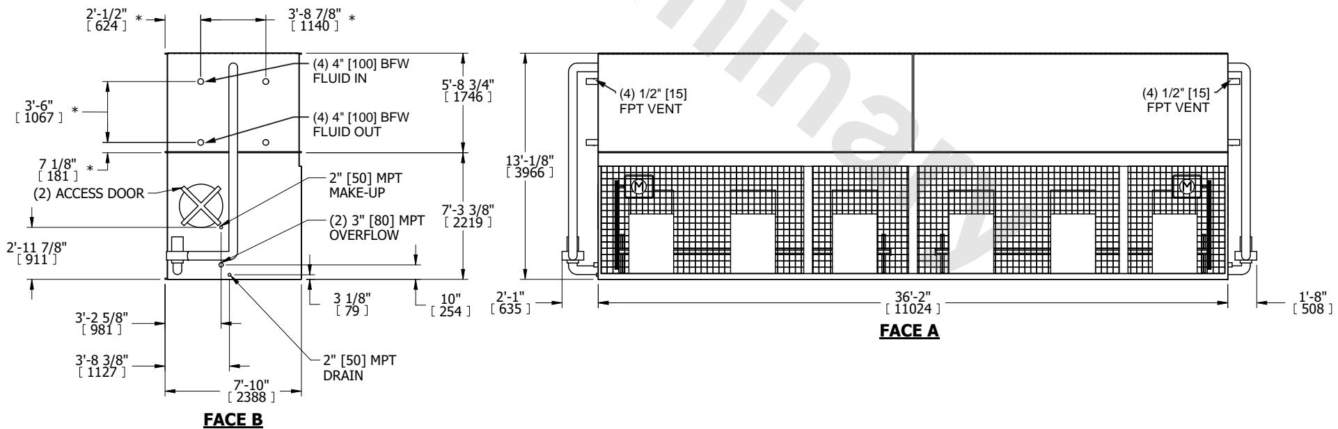
**SHIPPING WEIGHT** 50670 lbs+ [22985] kg+      **OPERATING WEIGHT** 70670 lbs+ [32060] kg+      **HEAVIEST SECTION WEIGHT** 20300 lbs+ [9210] kg+      **NO. OF SHIPPING SECTIONS** 3      **DRAWN BY:** TLS
