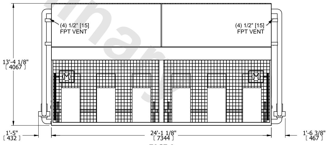
SHIPPING WEIGHT 34600 lbs+ [15695] kg+ OPERATING WEIGHT 49020 lbs+ [22240] kg+ HEAVIEST SECTION WEIGHT 12700 lbs+ [5765] kg+ NO. OF SHIPPING SECTIONS 3 DRAWN BY: TLS
