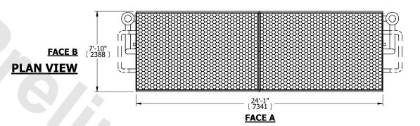
(4) 1/2" [15] (4) 1/2" [15] **FPT VENT** FPT VENT SERIES FLOW **PIPING** (BY OTHERS) (4) 4" [100] BFW **FLUID IN** 5'-1 1/4" [ 1556 ] AUX. CROSSOVER AUX. CROSSOVER DRAIN (BY OTHERS) DRAIN (BY OTHERS) 12'-4 5/8" (2) ACCESS DOOR (4) 4" [100] BFW FLUID OUT (2) 3" [80] MPT OVERFLOW 2" [50] MPT 7'-3 3/8" [ 2219 ] MAKE-UP 2'-11 7/8" [ 911 ] 24'-1" [ 7341 ] 10" [ 254 ] 1'-5" [ 432 ] 1'-6 5/8" 3'-2 5/8" [ 981 ] **FACE A** 3'-8 3/8" [ 1127 ] 2" [50] MPT DRAIN 7'-10" [ 2388 ] **FACE B**
