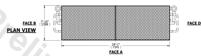
SERIES FLOW **PIPING** (4) 4" [100] BFW (BY OTHERS) (4) 1/2" [15] (4) 1/2" [15] FLUID IN FPT VENT **FPT VENT** 5'-8 3/4" (4) 4" [100] BFW AUX. CROSSOVER AUX. CROSSOVER FLUID OUT DRAIN (BY OTHERS) DRAIN (BY OTHERS) 13'-1/8" [ 3966 ] (2) ACCESS DOOR 2" [50] MPT (2) 3" [80] MPT MAKE-UP 7'-3 3/8" [ 2219 ] OVERFLOW 2'-11 7/8" [ 911 ] 1'-5" [ 432 ] 24'-1" [ 7341 ] 10" [ 254 ] **FACE A** 2" [50] MPT 7'-10" [ 2388 ] DRAIN
