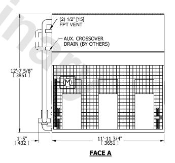
DRAWN BY: **SHIPPING** OPERATING NO. OF SHIPPING SECTIONS HEAVIEST SECTION 15130 lbs+ [6865] kg+ 21600 lbs+ [9800] kg+ 10080 lbs+ [4575] kg+ WEIGHT WEIGHT WEIGHT
