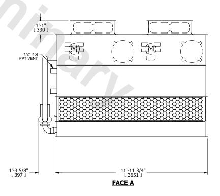
**SHIPPING** OPERATING HEAVIEST SECTION 5840 lbs+ [2650] kg+ 8740 lbs+ [3965] kg+ 5020 lbs+ [2280] kg+ WEIGHT WEIGHT WEIGHT
