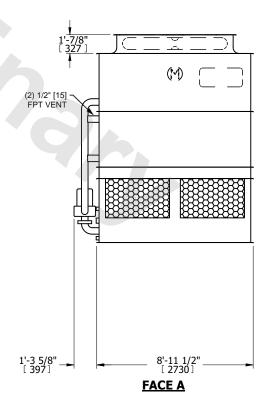
DRAWN BY: SLR NO. OF SHIPPING SECTIONS **SHIPPING OPERATING** HEAVIEST SECTION 11080 lbs+ [5030] kg+ 15480 lbs+ [7025] kg+ 9640 lbs+ [4375] kg+ WEIGHT WEIGHT WEIGHT
