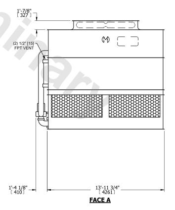
**SHIPPING** OPERATING HEAVIEST SECTION 18790 lbs+ [8525] kg+ 26410 lbs+ [11980] kg+ WEIGHT WEIGHT WEIGHT
