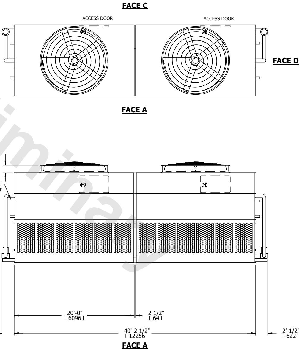
SHIPPING WEIGHT 64320 lbs+ [29180] kg+ OPERATING WEIGHT 96000 lbs+ [43545] kg+ HEAVIEST SECTION WEIGHT 27650 lbs+ [12545] kg+ NO. OF SHIPPING SECTIONS 4 DRAWN BY: SLR
