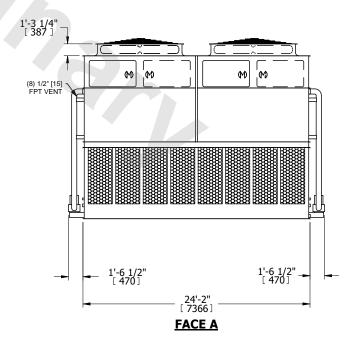
DRAWN BY: NO. OF SHIPPING SECTIONS **SHIPPING OPERATING** HEAVIEST SECTION 23760 lbs+ [10780] kg+ 106220 lbs+ [48185] kg+ 150480 lbs+ [68260] kg+ WEIGHT WEIGHT WEIGHT
