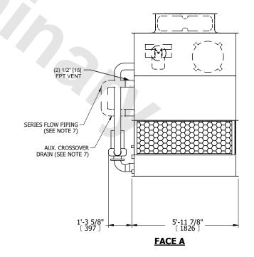
DRAWN BY: CAF NO. OF SHIPPING SECTIONS **SHIPPING** OPERATING HEAVIEST SECTION 3220 lbs+ [1465] kg+ 4740 lbs+ [2155] kg+ 2710 lbs+ [1230] kg+ WEIGHT WEIGHT WEIGHT
