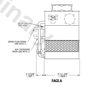
DRAWN BY: CAF NO. OF SHIPPING SECTIONS **SHIPPING OPERATING** HEAVIEST SECTION 3230 lbs+ [1470] kg+ 4750 lbs+ [2155] kg+ 2720 lbs+ [1235] kg+ WEIGHT WEIGHT WEIGHT
