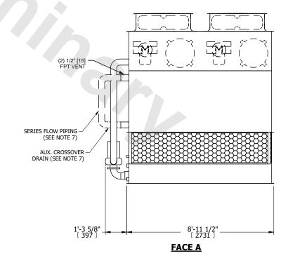
SHIPPING WEIGHT 6330 lbs+ [2875] kg+ OPERATING WEIGHT 8920 lbs+ [4050] kg+ HEAVIEST SECTION WEIGHT 5660 lbs+ [2570] kg+ NO. OF SHIPPING SECTIONS
