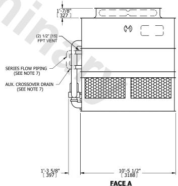
DRAWN BY: JLG NO. OF SHIPPING SECTIONS **SHIPPING** OPERATING HEAVIEST SECTION 9480 lbs+ [4305] kg+ 11120 lbs+ [5045] kg+ 15790 lbs+ [7165] kg+ WEIGHT WEIGHT WEIGHT
