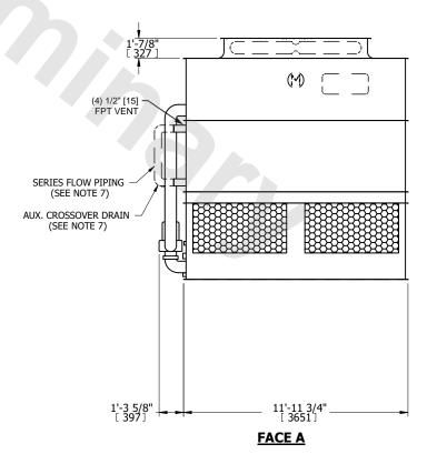
DRAWN BY: JLG NO. OF SHIPPING SECTIONS **SHIPPING** OPERATING HEAVIEST SECTION 16450 lbs+ [7465] kg+ 23000 lbs+ [10435] kg+ 14580 lbs+ [6615] kg+ WEIGHT WEIGHT WEIGHT
