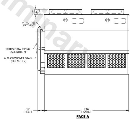
DRAWN BY: JLG NO. OF SHIPPING SECTIONS **SHIPPING** OPERATING HEAVIEST SECTION 25140 lbs+ [11405] kg+ 27930 lbs+ [12670] kg+ 38630 lbs+ [17525] kg+ WEIGHT WEIGHT WEIGHT
