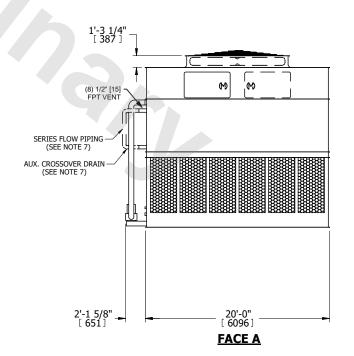
DRAWN BY: JLG **SHIPPING** OPERATING HEAVIEST SECTION NO. OF SHIPPING SECTIONS 86200 lbs+ [39100] kg+ 123320 lbs+ [55940] kg+ 38590 lbs+ [17505] kg+ WEIGHT WEIGHT WEIGHT
