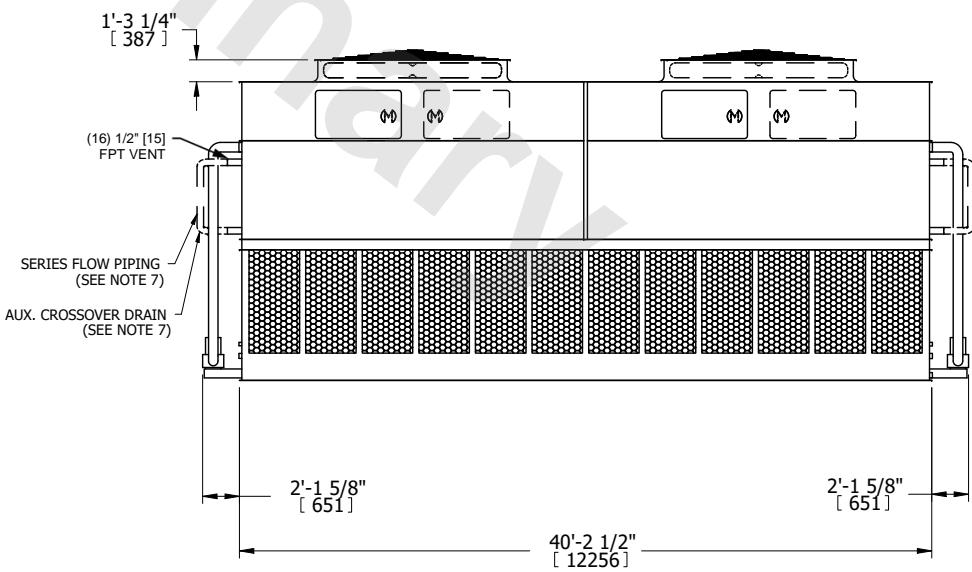
SHIPPING WEIGHT 172540 lbs+ [78265] kg+ OPERATING WEIGHT 246960 lbs+ [112020] kg+ HEAVIEST SECTION WEIGHT 38600 lbs+ [17510] kg+ NO. OF SHIPPING SECTIONS 6 DRAWN BY: JLG
