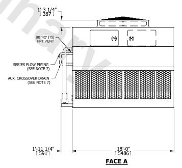
DRAWN BY: SLR **SHIPPING OPERATING** HEAVIEST SECTION NO. OF SHIPPING SECTIONS 41880 lbs+ [19000] kg+ 64440 lbs+ [29230] kg+ 17270 lbs+ [7835] kg+ WEIGHT WEIGHT WEIGHT
