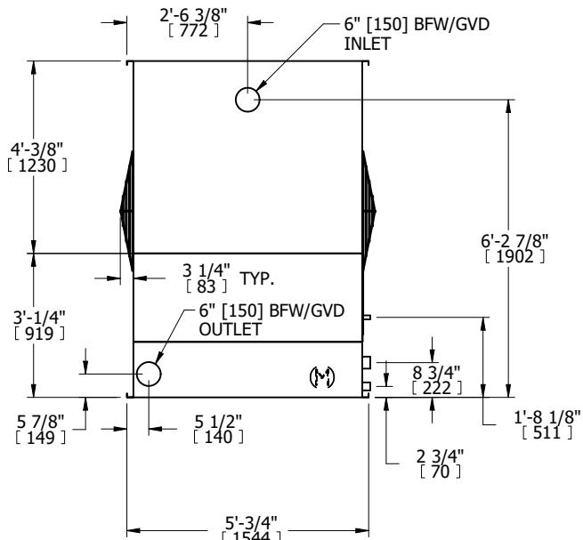
SHIPPING WEIGHT 2990 lbs+ [1360] kg+ OPERATING WEIGHT 5590 lbs+ [2540] kg+ HEAVIEST SECTION WEIGHT 2990 lbs+ [1360] kg+ NO. OF SHIPPING SECTIONS 1 DRAWN BY: JLG
