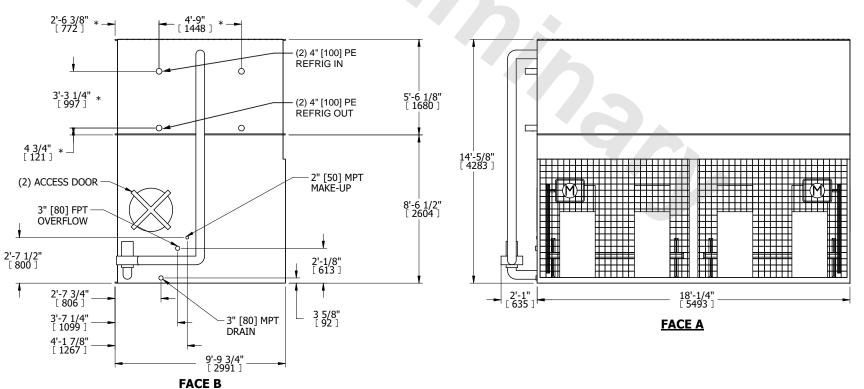
DRAWN BY: NO. OF SHIPPING SECTIONS **SHIPPING** OPERATING HEAVIEST SECTION 24240 lbs+ [11000] kg+ 17050 lbs+ [7735] kg+ 32020 lbs+ [14525] kg+ WEIGHT WEIGHT WEIGHT
