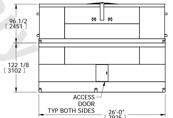
SHIPPING WEIGHT 74300 lbs+ [33705] kg+ OPERATING WEIGHT 116140 lbs+ [52685] kg+ HEAVIEST SECTION WEIGHT 25650 lbs+ [11635] kg+ NO. OF SHIPPING SECTIONS 4 DRAWN BY: TLS
