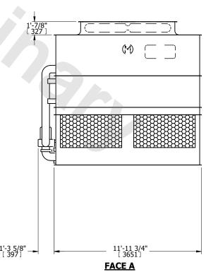
**SHIPPING OPERATING** HEAVIEST SECTION 10150 lbs+ [4605] kg+ 12020 lbs+ [5455] kg+ 16060 lbs+ [7285] kg+ WEIGHT WEIGHT WEIGHT
