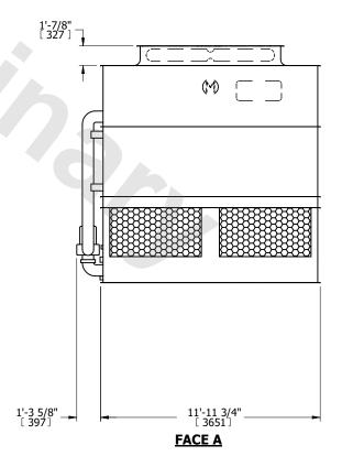
DRAWN BY: SLR NO. OF SHIPPING SECTIONS **SHIPPING** OPERATING HEAVIEST SECTION 16240 lbs+ [7370] kg+ 14370 lbs+ [6520] kg+ 20540 lbs+ [9320] kg+ WEIGHT WEIGHT WEIGHT
