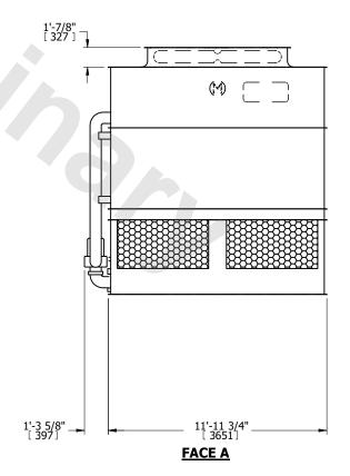
DRAWN BY: SLR NO. OF SHIPPING SECTIONS **SHIPPING** OPERATING HEAVIEST SECTION 18490 lbs+ [8390] kg+ 16620 lbs+ [7540] kg+ 22910 lbs+ [10395] kg+ WEIGHT WEIGHT WEIGHT
