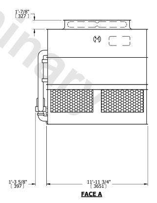
DRAWN BY: SLR NO. OF SHIPPING SECTIONS **SHIPPING** OPERATING HEAVIEST SECTION 14210 lbs+ [6450] kg+ 12340 lbs+ [5600] kg+ 18380 lbs+ [8340] kg+ WEIGHT WEIGHT WEIGHT
