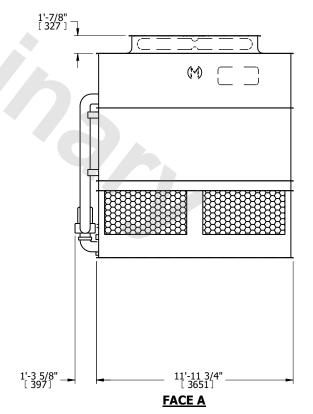
DRAWN BY: SLR NO. OF SHIPPING SECTIONS **SHIPPING OPERATING** HEAVIEST SECTION 18710 lbs+ [8490] kg+ 16840 lbs+ [7640] kg+ 23130 lbs+ [10495] kg+ WEIGHT WEIGHT WEIGHT
