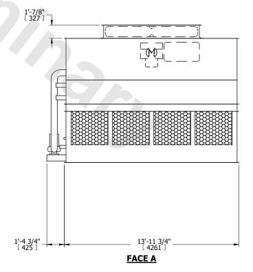
DRAWN BY: JLG NO. OF SHIPPING SECTIONS **SHIPPING** OPERATING HEAVIEST SECTION 11100 lbs+ [5035] kg+ 9020 lbs+ [4095] kg+ 15650 lbs+ [7100] kg+ WEIGHT WEIGHT WEIGHT
