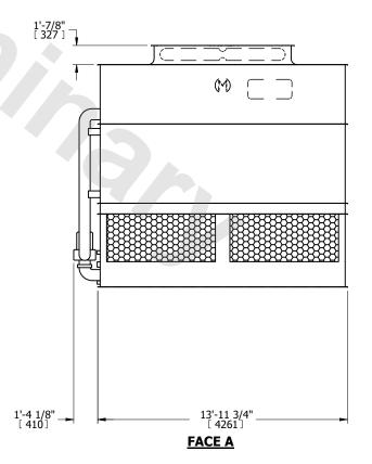
DRAWN BY: SLR NO. OF SHIPPING SECTIONS **SHIPPING** OPERATING HEAVIEST SECTION 21300 lbs+ [9665] kg+ 19220 lbs+ [8720] kg+ 26440 lbs+ [11995] kg+ WEIGHT WEIGHT WEIGHT
