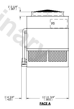
SHIPPING WEIGHT 26520 lbs+ [12030] kg+ OPERATING WEIGHT 33680 lbs+ [15280] kg+ HEAVIEST SECTION WEIGHT 23810 lbs+ [10805] kg+ NO. OF SHIPPING SECTIONS
