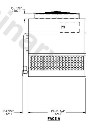
DRAWN BY: SLR NO. OF SHIPPING SECTIONS **SHIPPING** OPERATING HEAVIEST SECTION 26560 lbs+ [12050] kg+ 23500 lbs+ [10660] kg+ 34780 lbs+ [15780] kg+ WEIGHT WEIGHT WEIGHT
