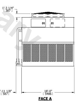
SHIPPING WEIGHT 67480 lbs+ [30610] kg+ OPERATING WEIGHT 88520 lbs+ [40155] kg+ HEAVIEST SECTION WEIGHT 29820 lbs+ [13530] kg+ NO. OF SHIPPING SECTIONS 4 DRAWN BY: SLR
