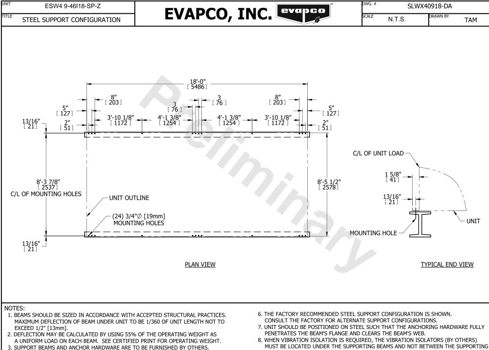
3. SUPPORT BEAMS AND ANCHOR HARDWARE ARE TO BE FURNISHED BY OTHERS ANCHOR HARDWARE TO BE ASTM A325 5/8" [16mm] BOLT OR EQUIVALENT.
