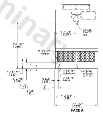
SHIPPING WEIGHT 3700 lbs+ [1680] kg+ OPERATING WEIGHT 5740 lbs+ [2605] kg+ HEAVIEST SECTION WEIGHT 2570 lbs+ [1170] kg+ NO. OF SHIPPING SECTIONS 2
